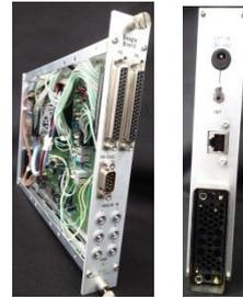
Figure 6: BBB installed in NIM chassis. 60 bit Digital I/O, 1 port RS232C, 6 channels ADC are available.
